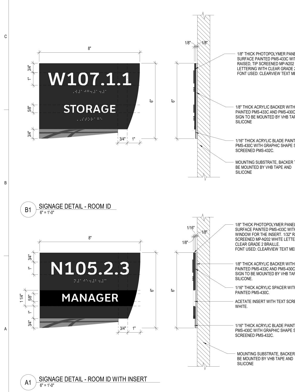
1/8" THICK PHOTOPOLYMER PANEL SECOND SURFACE PAINTED PMS-433C WITH 1/32" RAISED, TIP SCREENED MP-N202 WHITE LETTERING WITH CLEAR GRADE 2 BRAILLE. FONT USED: CLEARVIEW TEXT MEDIUM
