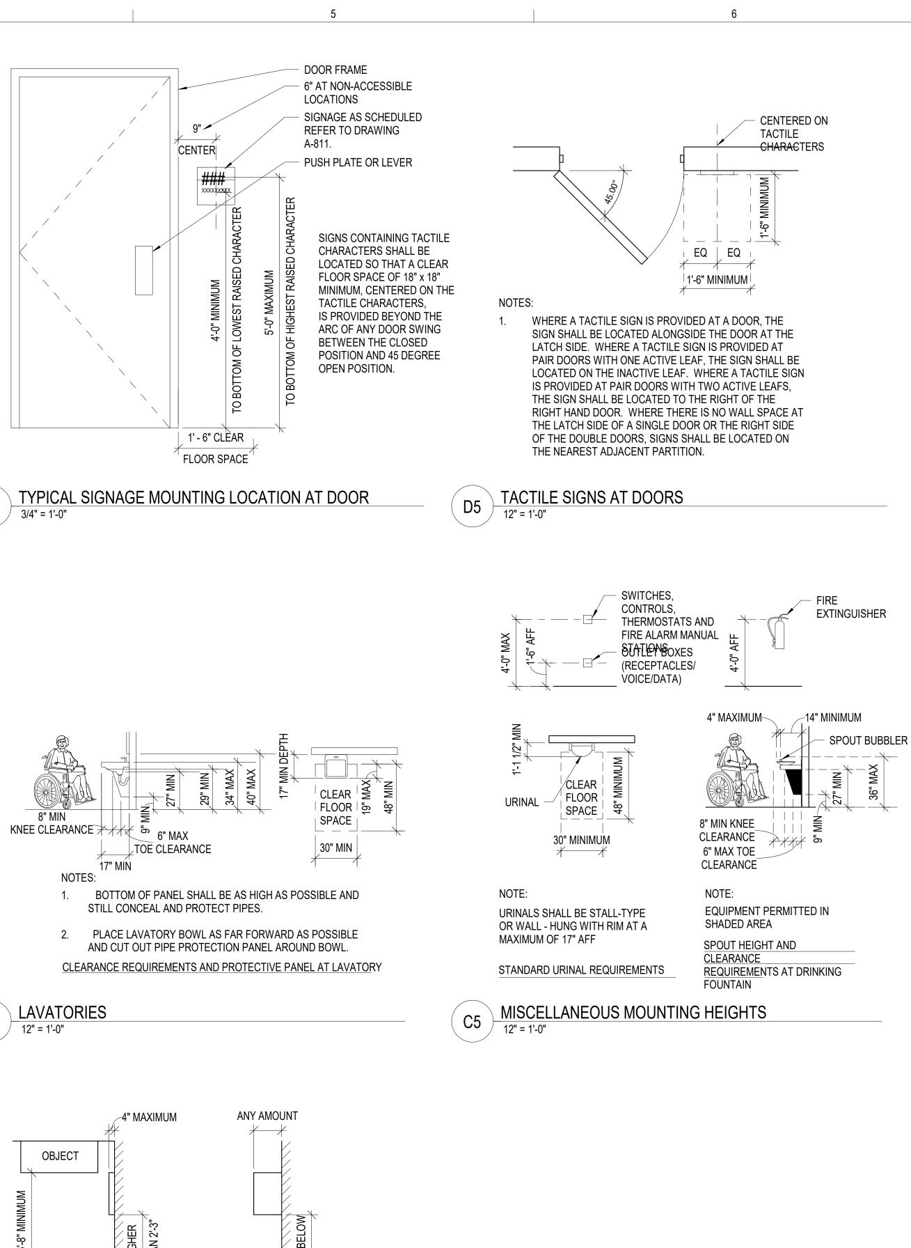
1. OBJECTS PROJECTING FROM WALLS WHOSE LEADING EDGES ARE BETWEEN 27" AND 80" ABOVE FINISH FLOOR SHALL NOT PROTRUDE MORE THAN 4" INTO WALKS, WALLS, CORRIDORS, PASSAGEWAYS, OR AISLES.
