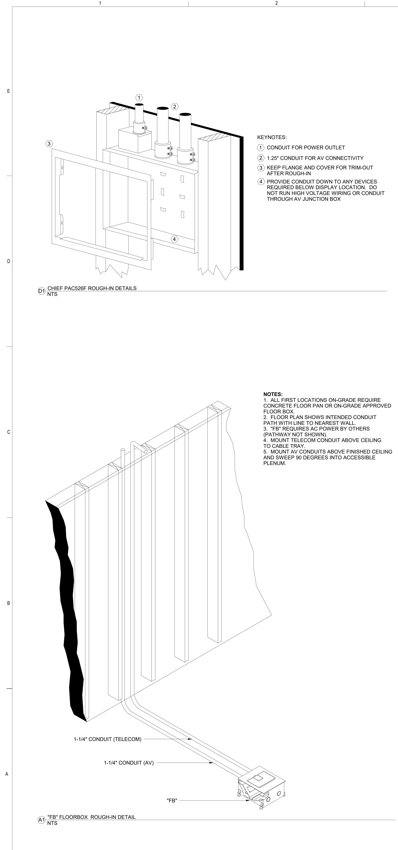
$\langle 2 \rangle$  1.25" CONDUIT FOR AV CONNECTIVITY  $\langle \underline{\mathbf{3}} \rangle$  KEEP FLANGE AND COVER FOR TRIM-OUT AFTER ROUGH-IN
